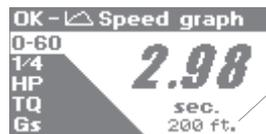
The 60-0 MPH braking distance is shown below the 0-60 MPH time if the run was completed by braking hard to a complete stop, and then waiting for the E.T. clock to stop.
