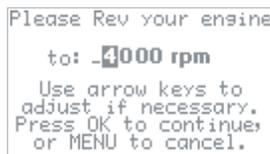
If you would like to calibrate at 6000 RPMs instead of 4000 RPMs, just press **▲** twice to change the “4000” to a “6000”, and then rev your engine to 6000 RPMs and press **OK**.
